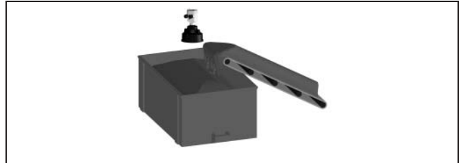
Fig. 2: Level measurement in a container with VEGASON 63
