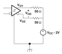
Figure 39. Typical Termination for LVPECL Output Driver (SN65LVDx101)
