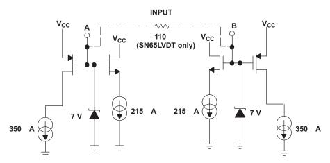
Figure 38. Receiver Equivalent Schematic
