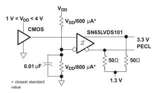
Figure 49. Single-Ended CMOS to 3.3-V PECL Translation
