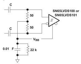
Figure 50. Receipt of AC-Coupled Signals
