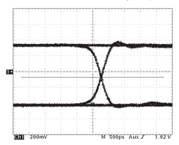
Figure 37. Receiver Input Eye Pattern with External Failsafe
