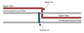
Figure 57. Ground Via Location (Side View)
