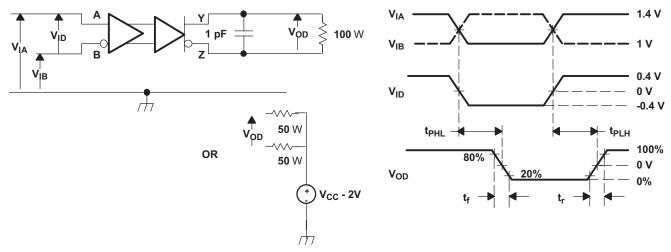
NOTE: All input pulses are supplied by a generator having the following characteristics:  $t_r$  or  $t_f \le 0.25$  ns, pulse repetition rate (PRR) = 50 Mpps, pulse width = 10 ± 0.2 ns.  $C_L$  includes instrumentation and fixture capacitance within 0.06 mm of the device under test. Measurement equipment provides a bandwidth of 5 GHz minimum.
