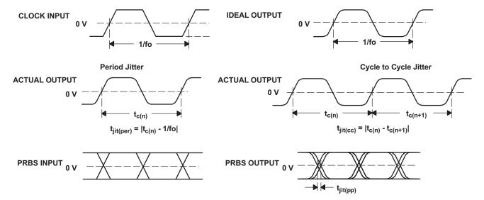
Figure 34. Driver Jitter Measurement Waveforms
