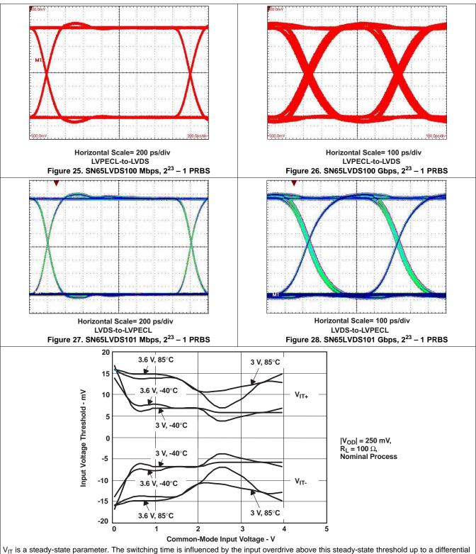
V<sub>IT</sub> is a steady-state parameter. The switching time is influenced by the input overdrive above this steady-state threshold up to a differentia input voltage magnitude of 100 mV.
