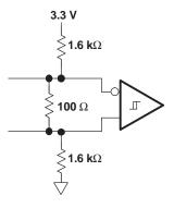
Figure 36. External Failsafe Circuit
