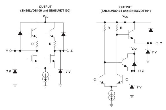
Figure 40. Driver Equivalent Schematics
