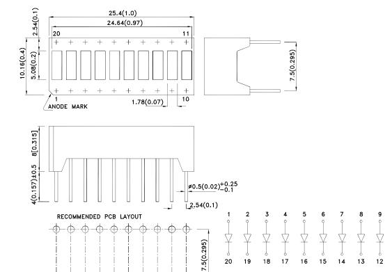
1. All dimensions are in millimeters (inches), Tolerance is ±0.25(0.01")unless otherwise noted.
