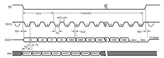
Figure 3. ADC104S051 Serial Timing Diagram
