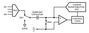
Figure 47. ADC104S051 in Track Mode
