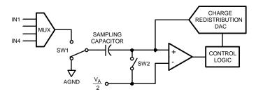
Figure 48. ADC104S051 in Hold Mode
