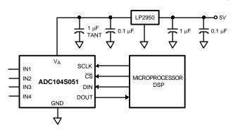
Figure 50. Typical Application Circuit
