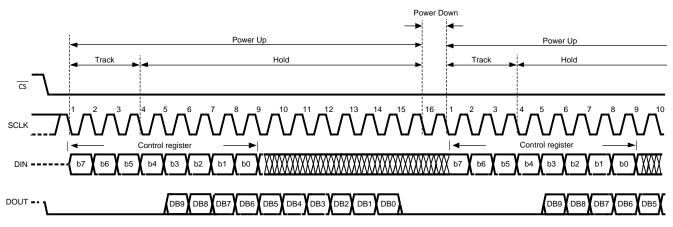
Figure 1. ADC104S051 Operational Timing Diagram
