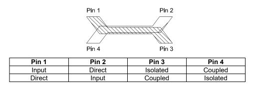
Note: The direct port has a DC connection to the input port and the coupled port has a DC connection to the isolated port.
