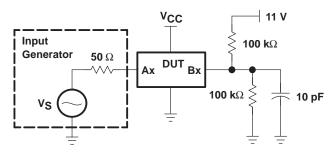
Figure 1. Device Test Setup
