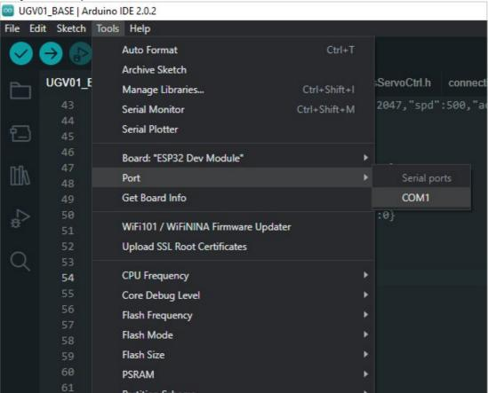
4. Connect the driver board to the computer with a USB cable, then click Tools -> Ports, select uf2 Board for the first connection, and after the upload is complete, connecting again will result in an additional COM port.
