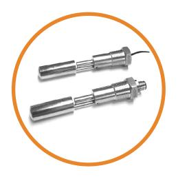
The SSF215 series of floatswitches are externally mounted horizontal switches. This series has an extended reach to provide a solution for extra thick tank walls or for mounting in welded on 1/2"NPT bosses.
