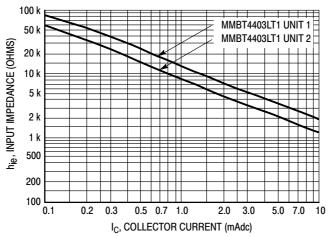
Figure 9. Input Impedance
