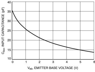
Figure 18. Input Capacitance vs. Emitter Base . Voltage
