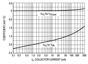
Figure 15. Temperature Coefficients
