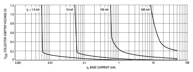
Figure 13. Collector Saturation Region
