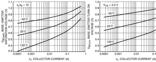
Figure 16. Base-Emitter Saturation Voltage vs. **Collector Current**
