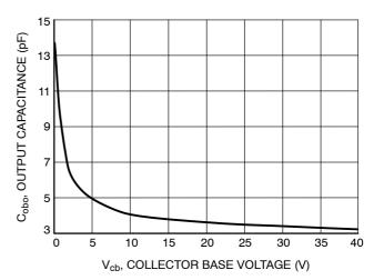
Figure 19. Output Capacitance vs. Collector Base Voltage
