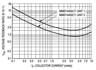
Figure 10. Voltage Feedback Ratio
