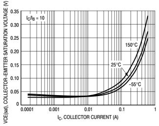
Figure 14. Collector-Emitter Saturation Voltage vs. Collector Current
