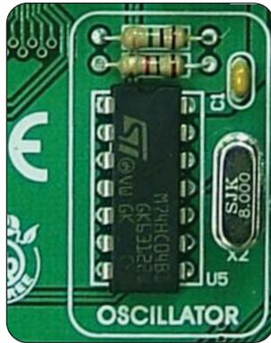
Figure 13 On-board oscillator
