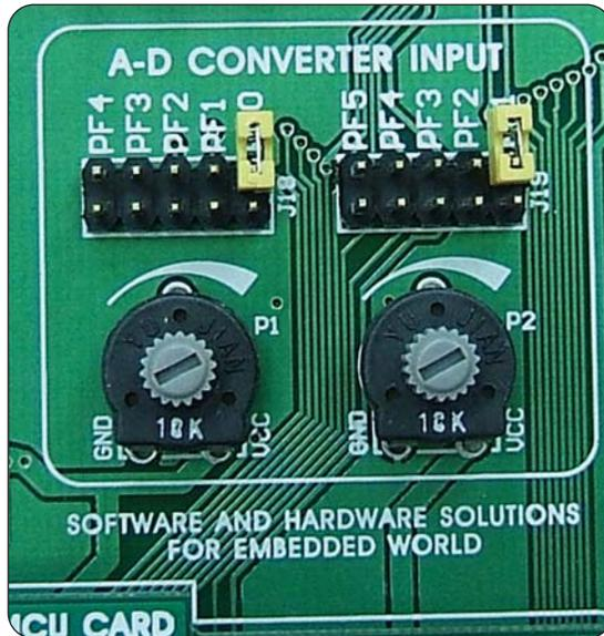
**Figure 34** A/D converter inputs
