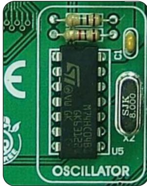
Figure 13 On-board oscillator
