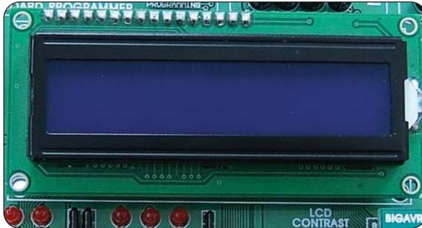
**Figure 24** 2x16 LCD in 4-bit mode
