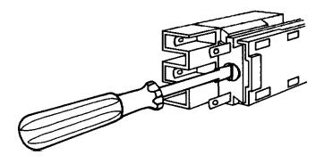
Securing: By a quarer-turn to the right of the red locking pin (with a screwdriver),
