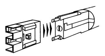
Assembly: The contact block is a sliding fit onto the dovetailed switch body; turn the nick of the red locking pin parallel to the dovetail.
