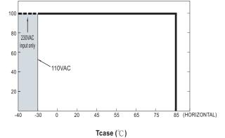
$\odot$  If ELG-300 operates in Constant Current mode with the rated current, the maximum workable Ta is 40 $^{\circ}$ C.
