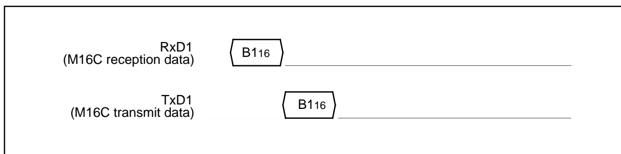
Figure 1.32.39. Timing of baud rate 19200
