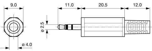
Cable diameter max. 4.0 mm
