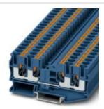
Feed-through terminal block, Connection method: Push-in connection, Cross section: 0.5 mm² - 10 mm², AWG: 20 - 8, Width: 8.2 mm, Height: 42.2 mm, Color: gray, Mounting type: NS 35/7,5, NS 35/15
