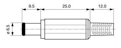
Cable diameter max. 4.0 mm
