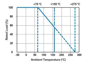
For resistors operated in ambient temperatures above  $70^{\circ}$ C, power rating must be derated in accordance with this curve.
