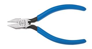
These Klein Tools 5-Inch Electronics Pliers have a narrow jaw and hinge with a sharp, pointed nose for precise tip cutting and trimming of printed circuit boards. Made of US-made steel and induction hardened for long life. Spring assisted, hot-riveted joint for a smooth action and no wobble handle. The handles are plastic dipped for comfort and ease of identification.
