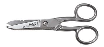
These Klein Tools Cable Splicer Snips cut 19 AWG and 23 AWG electrical wire, cable and cordage. The stainless steel blades maintain sharpness and durability. Serrated teeth provide non-slip cutting action. The snip has a free-fall feature for ease of use.
