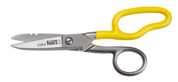
These Scissors are free-fall snips that feature stainless steel blades for blade sharpness and durability. They cut 19 AWG and 23 AWG electrical communication wire, cable and cordage. The extended handle allows for more comfortable cutting and provides leverage during wire cutting. The free-fall design makes this snip easier to use.
