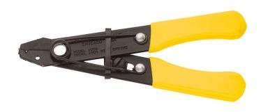
Klein Tools 1004 Wire Stripper and Cutter is a handy, light, compact tool for stripping insulation. Spring-loaded for action for self-opening. Convenient hole for looping or bending wire. Adjustable slide stop with set screw for repeat stripping work.
