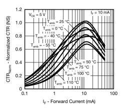
Fig. 11 - Normalized CTR (NS) vs. Forward Current
