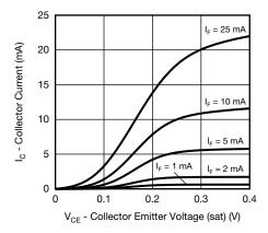
Fig. 7 - Collector Current vs. Collector Emitter Voltage (sat)
