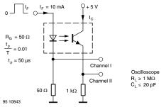
Fig. 3 - Test Circuit, Saturated Operation
