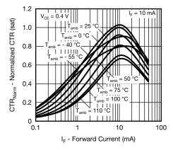
Fig. 12 - Normalized CTR (sat) vs. Forward Current
