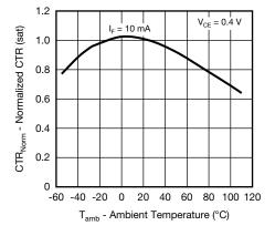
Fig. 10 - Normalized CTR (sat) vs. Ambient Temperature
