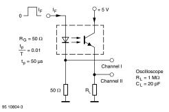
Fig. 2 - Test Circuit, Non-Saturated Operation
