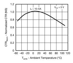
Fig. 9 - Normalized CTR (NS) vs. Ambient Temperature
