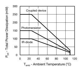
Fig. 1 - Total Power Dissipation vs. Ambient Temperature
