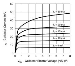
Fig. 6 - Collector Current vs. Collector Emitter Voltage (NS)
