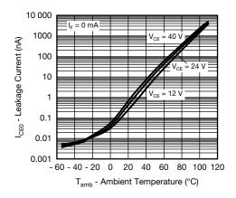
Fig. 8 - Leakage Current vs. Ambient Temperature
