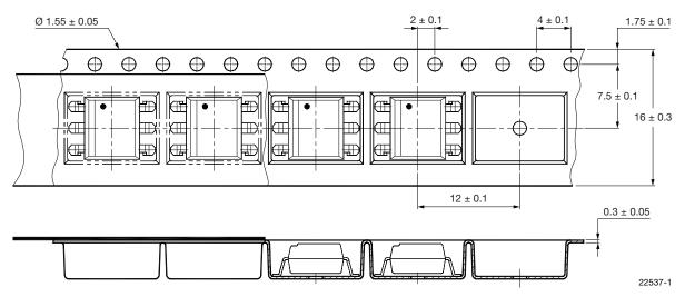
Fig. 16 - Tape and Reel Drawing, 1000 Units per Reel
