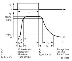
Fig. 4 - Switching Times
