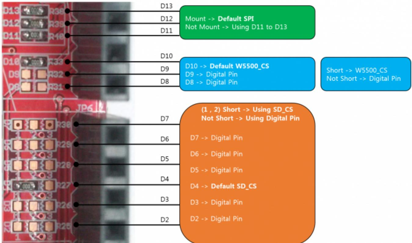
W5500 Ethernet shield has several configurable GPIOs
