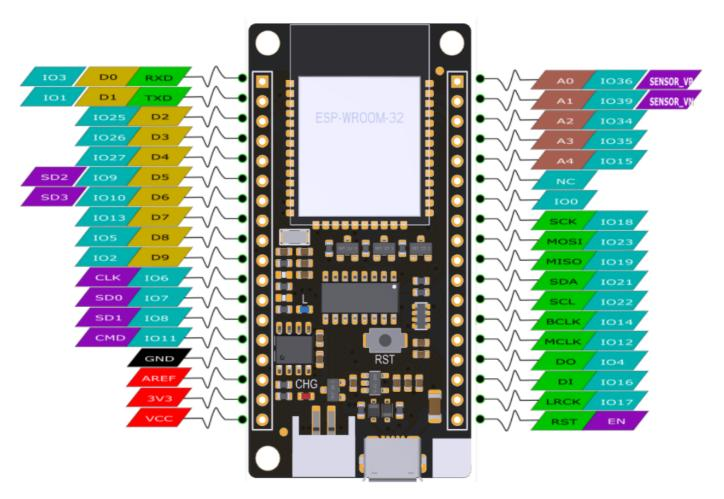
**NOTE**: NC = Empty; VCC = VCC (5V under USB power supply, Around 3.7V under 3.7V lipo battery.power supply)
