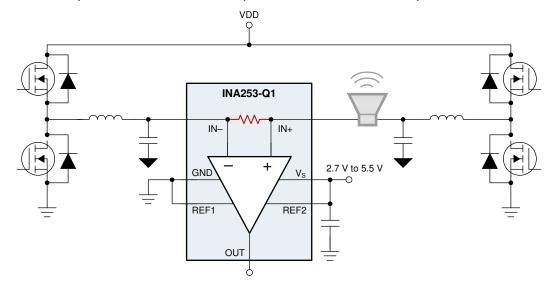
Figure 8-5. Current Sensing in a CLASS-D Subsystem
