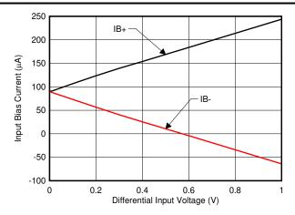
Figure 8-2. Input Bias Current vs Differential Input Voltage
