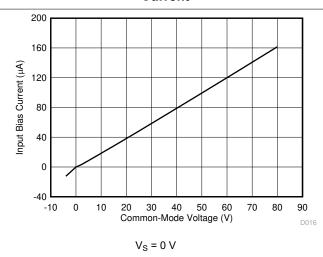
Figure 6-16. Input Bias Current vs Common-Mode Voltage
