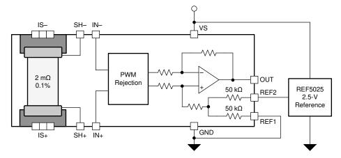
Figure 7-9. Mid-External Reference Output
