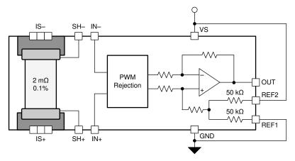
Figure 7-8. Mid-Supply Voltage Output
