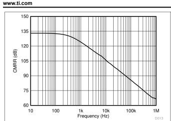
Figure 6-13. Common-Mode Rejection Ratio vs Frequency
