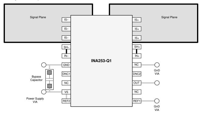
Figure 10-1. INA253-Q1 Layout Example
