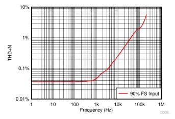
Figure 7-4. Amplifier Performance Over Frequency
