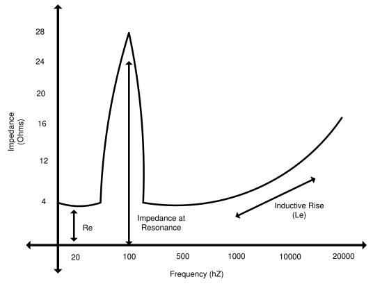
Figure 8-6. Speaker Impedance Measurement
