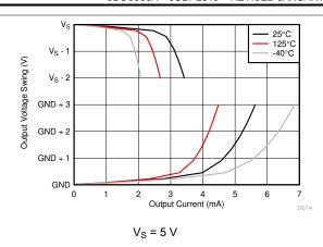
Figure 6-14. Output Voltage Swing vs Output Current
