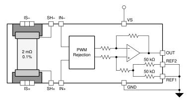
Figure 7-6. Ground-Referenced Output
