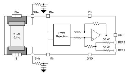
Figure 8-1. Filter at Input Pins
