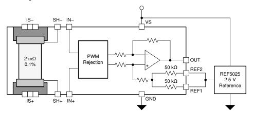
Figure 7-7. External Reference Output
