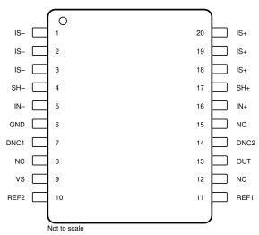
Figure 5-1. PW Package 20-Pin TSSOP Top View
