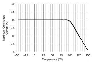
Figure 7-1. Maximum Continuous Current vs Temperature
