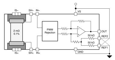
Figure 7-5. Adjusting the Output Midpoint
