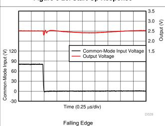
Figure 6-28. Common-Mode Voltage Transient Response
