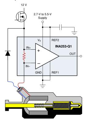
Figure 8-3. Solenoid Drive Application Circuit
