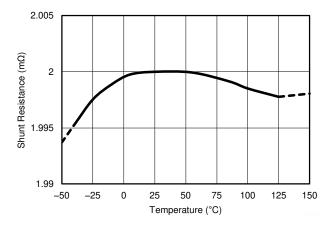
Figure 7-3. Sensing Resistor vs Temperature
