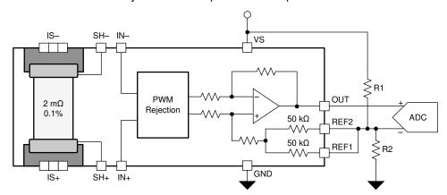
Figure 7-10. Setting the Reference Using a Resistor Divider
