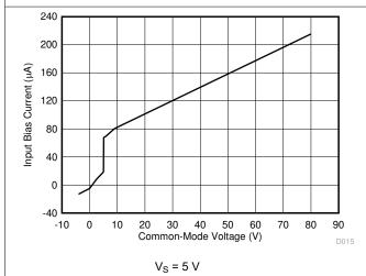
Figure 6-15. Input Bias Current vs Common-Mode Voltage
