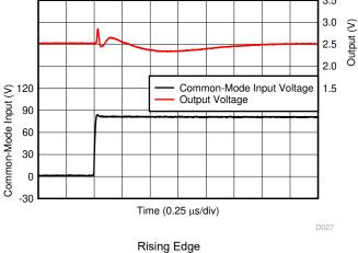
Figure 6-27. Common-Mode Voltage Transient Response
