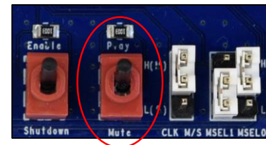
Figure 11. Right toggle switch set to “play” position.
