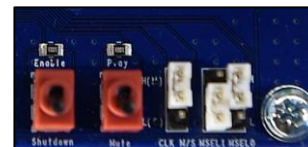
Figure 6. Toggle buttons set to “mute” and “shutdown”
