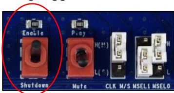
Figure 8. Left toggle switch set to “enable” position.
