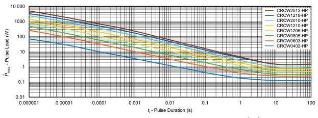
Maximum pulse load, single pulse; applicable if  $\bar{P} \rightarrow 0$  and n < 1000 and  $\hat{U} \le \hat{U}_{max}$ ; for permissible resistance change equivalent to 8000 h operation
