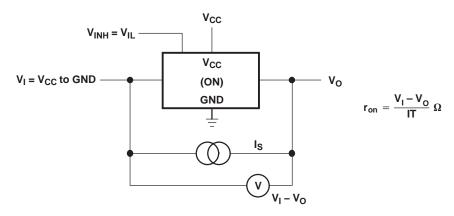
Figure 5. On-State Resistance Test Circuit
