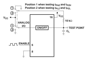
Figure 14. Propagation Delay, Enable to Analog Out, Test Setup
