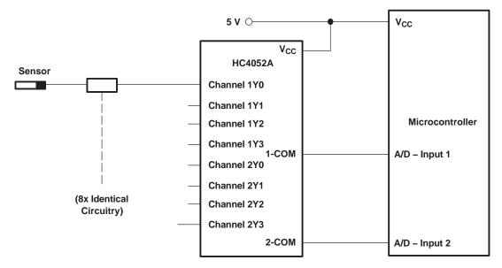
Figure 3. Solution by Applying the HC4852 Multiplexer
