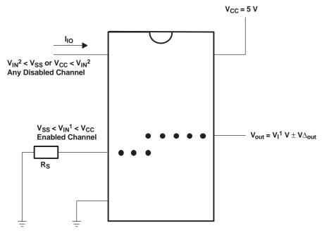
Figure 1. Injection-Current Coupling Specification
