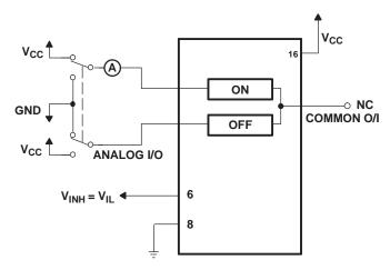
Figure 8. Maximum On-Channel Leakage Current, Channel to Channel, Test Setup
