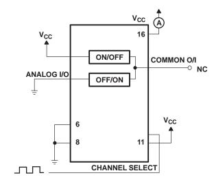
Figure 15. Power-Dissipation Capacitance, Test Setup
