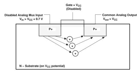
Figure 4. Diagram of Bipolar Coupling Mechanism (Appears if  $V_{IN}$  Exceeds  $V_{CC}$ , Driving Injection Current Into the Substrate)
