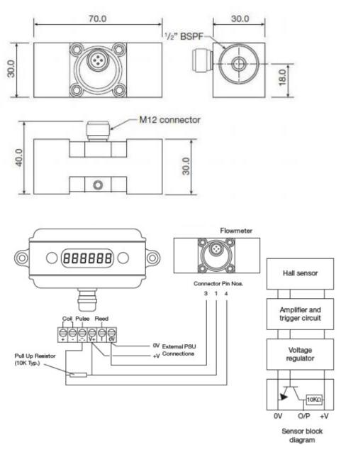
At the heart of the turbine flow meter is a precision turbine that rotates freely on robust sapphire bearings and contains over-moulded magnets that are detected through the chamber wall by a Hall effect detector. The output is a stream of NPN pulses that readily interfaces with most electronic display or recording devices. This combination of materials and technology ensures a long life product with reliable operation throughout. Viton 'O'Rings and 316 St St body and cap.
