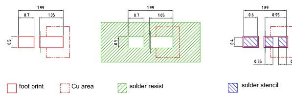
The usage of solder resist between anode and cathode pads is mandatory for applications where water may condense
