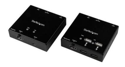
This HDMI® extender kit lets you transmit your 1080p HD video source to your remote HDMI display at distance of up to 165 ft. away (50 m) using shielded CAT6 cabling. The extender features a built-in 4-port USB 2.0 hub that also lets you connect four remote USB peripheral devices at your display location.
