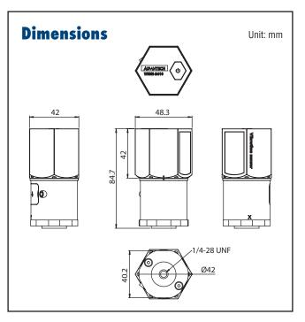
Stud mount, Mounting pad and Adhesives 84.7 x 48.3 mm CE (RED), FCC, NCC, TELEC, VCCI, BSMI, RCM, ANATEL
