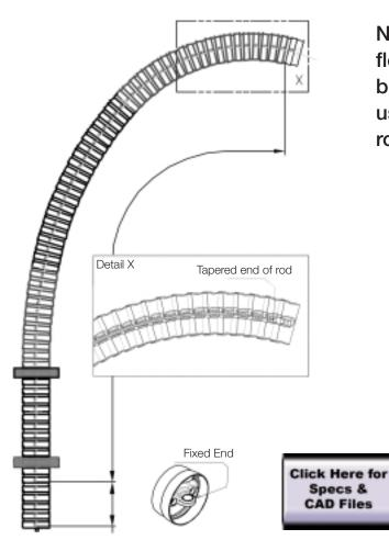
NOTE: Fiber rod segments will flex ONLY, not bend. Fiber rod will break if bent too much. Always use additional links after a fiber rod segment.
