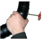
3. Push screwdriver through perforated window, moving chain links to the maximum bending position on the opposite side
