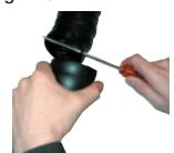
Remove socket from ball using the screwdriver as a lever.
