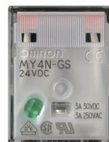
Relay with DC Coil (LED: Green)
