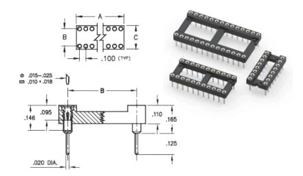
**Description:** DIP Dual In Line Socket Standard Solder Tail Open Frame Through Hole Plating Code:
