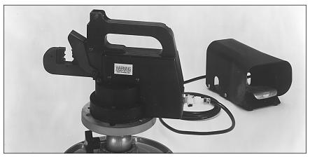
The Amphenol pneumatic crimp tool 227-60 is designed for use in high volume RF connector/cable assembly applications. Bench mountable on a swivel base, this high speed crimp tool runs on a standard 85/100 psi airline and is actuated by a foot switch for hands-free operation.
