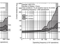
The tests were conducted at an ambient temperature of 23°C. The contact resistance data are periodically measured reference values \*2. and are not values from each monitoring operation. Contact resistance values will vary according to the switching frequency and operating environment, so be sure to check operation under the actual operating conditions before use.
