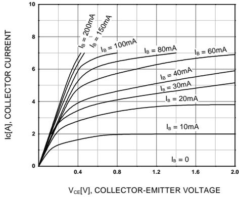
Figure 1. Static Characteristic
