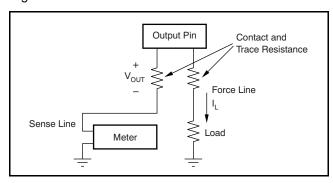
Figure 98. Accurate Load Regulation of the DAC8564 Internal Reference
