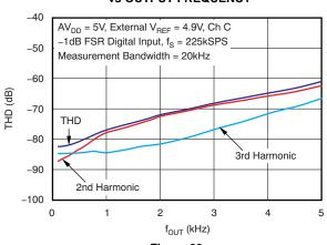
**TOTAL HARMONIC DISTORTION vs OUTPUT FREQUENCY**
