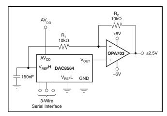
Figure 100. Bipolar Output Range Using Internal Reference
