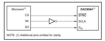
Figure 102. DAC8564 to Microwire Interface
