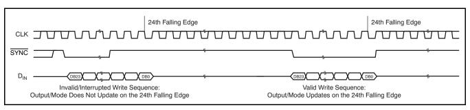
Figure 95. SYNC Interrupt Facility
