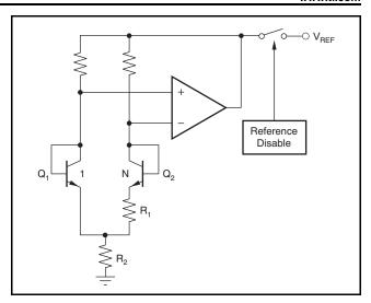
Figure 94. Simplified Schematic of the Bandgap Reference
