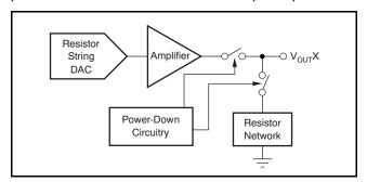
Figure 96. Output Stage During Power-Down
