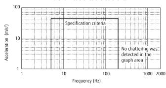
Test material: coil energized and de-energized Direction of vibration: see diagram below Detection level: chatter >1 ms
