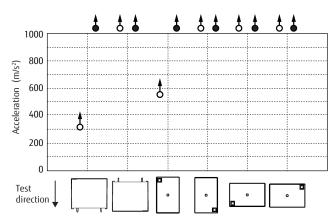
Test material: coil energized and de-energized Shock duration: 11ms (490m/s<sup>2</sup> or less)
