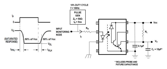
Figure 15: Test Circuit for Transient Immunity and Typical Waveforms
