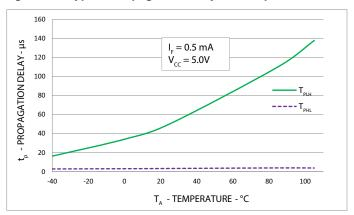
Figure 11: Typical Propagation Delay vs. Temperature
