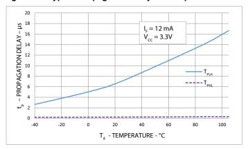
Figure 13: Typical Propagation Delay vs. Temperature
