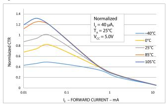
Figure 5: Current Transfer Ratio vs Forward Current
