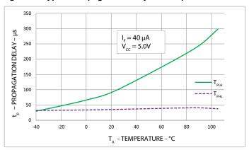
Figure 9: Typical Propagation Delay vs. Temperature
