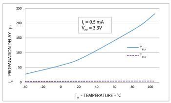
Figure 12: Typical Propagation Delay vs. Temperature
