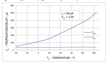
Figure 10: Typical Propagation Delay vs. Temperature
