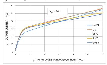
Figure 7: Logic Low Output Current vs. Temperature
