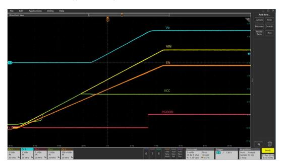
Figure 3 Startup with no load (Ch1:PV<sub>IN</sub>, Ch2: V<sub>OUT</sub>, Ch3: PG, Ch4:V<sub>CC</sub>, Ch5: Enable)
