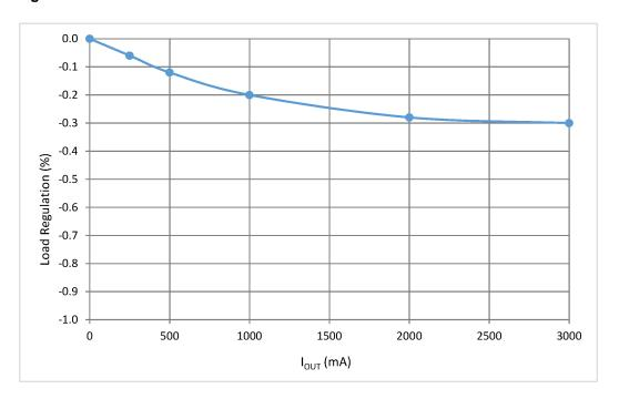
Figure 16 Load regulation ( $I_{0} = 0-3A$ )
