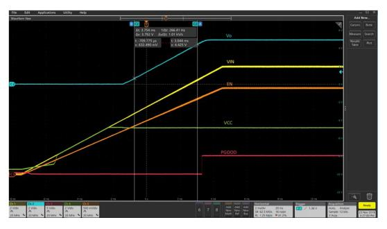
Figure 4 Startup with 3A load (Ch1:PV<sub>IN</sub>, Ch2: V<sub>OUT</sub>, Ch3: PG, Ch4:V<sub>CC</sub>, Ch5: Enable)
