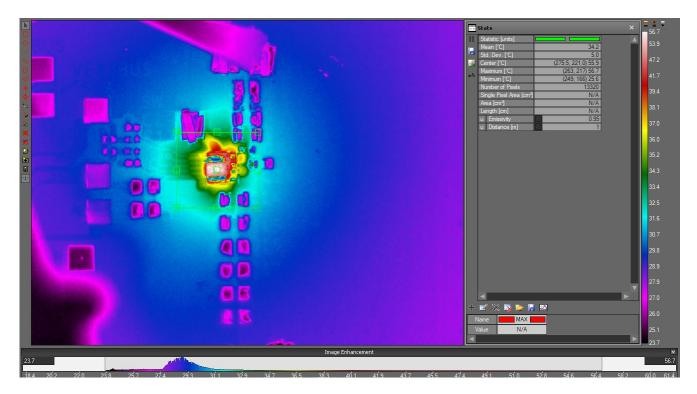
Figure 17 Thermal image – maximum temperature reached by FS1403 = 56.7°C
