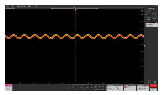
Figure 11  $V_{OUT}$  ripple 30mV at 0A (Ch7: $V_{OUT}$ )
