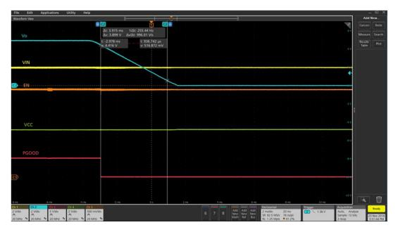
Figure 6 Soft turn off at 3A (Ch1:PV<sub>IN</sub>, Ch2: V<sub>OUT</sub>, Ch3: PG, Ch4:V<sub>CO</sub>, Ch5: Enable)
