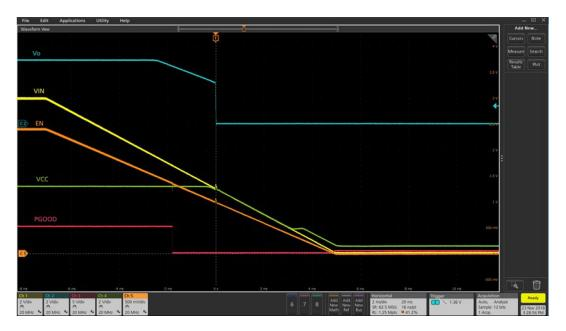
Figure 5 Shutdown with Enable de-assertion at 3A load (Ch1:PV<sub>IN</sub>, Ch2: V<sub>OUT</sub>, Ch3: PG, Ch4:V<sub>CC</sub>, Ch5: Enable)
