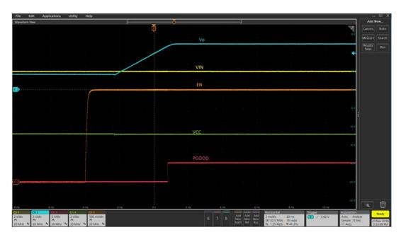
Figure 7 Startup into pre-bias (Ch1:PV<sub>IN</sub>, Ch2: V<sub>OUT</sub>, Ch3: PG, Ch4:V<sub>CC</sub>, Ch5: Enable)
