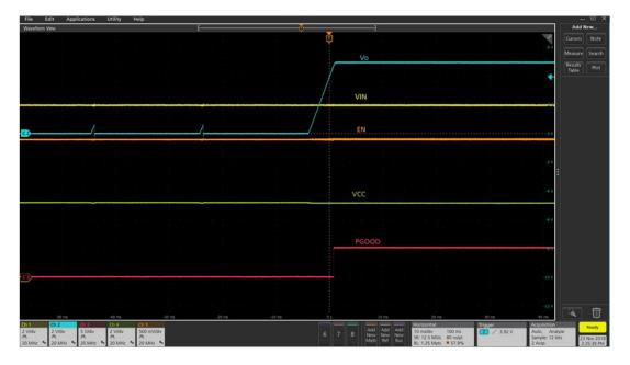
Figure 8 Over-current protection and auto-recover to 3A (Ch1:PV<sub>IN</sub>, Ch2:  $V_{OUT}$ , Ch3: PG, Ch4: $V_{CG}$ , Ch5: Enable)
