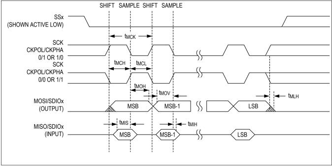
Figure 1. SPI Master Mode Timing Diagram
