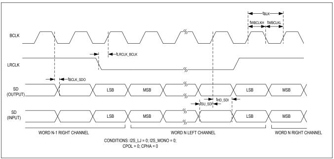
Figure 4. I<sup>2</sup>S Timing Diagram
