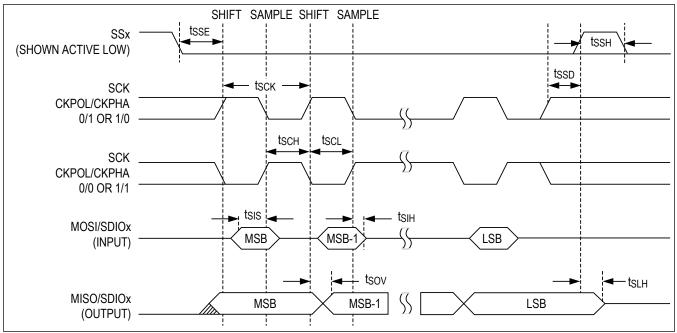
Figure 2. SPI Slave Mode Timing Diagram
