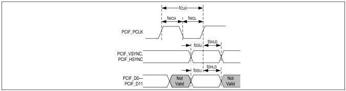
Figure 5. Parallel Camera Interface Timing Diagram
