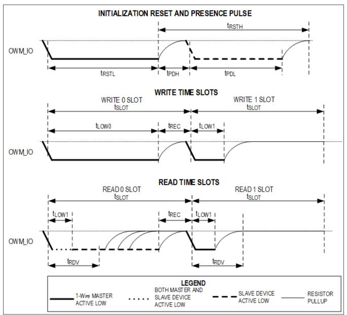
Figure 6. 1-Wire Master Data Timing Diagram
