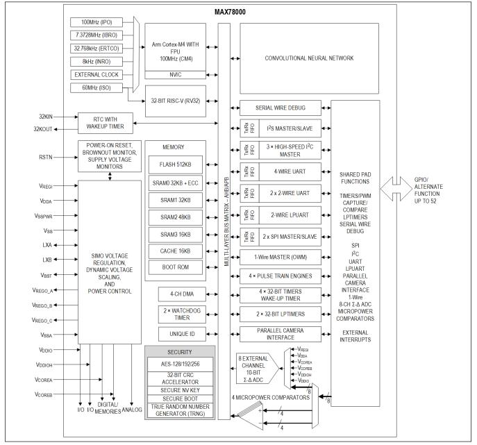
Ultra-Low-Power Arm Cortex-M4 Processor with FPU-Based Microcontroller with Convolutional Neural Network Accelerator
