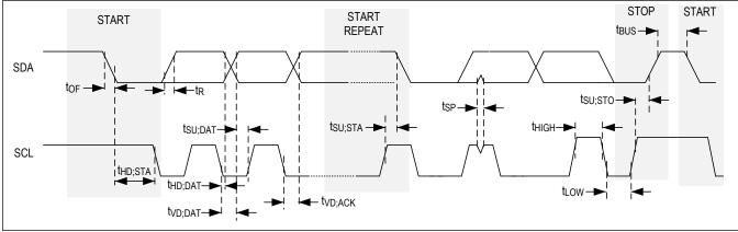
Figure 3. I<sup>2</sup>C Timing Diagram
