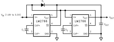
Figure 13. Lowering Output Resistance By Paralleling Devices
