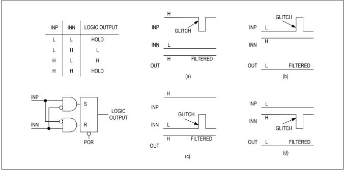
Figure 5. MAX2270\_D Differential Inputs
