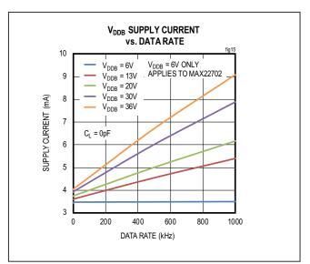
Figure 15. V<sub>DDB</sub> Supply Current vs. Data Rate (typ)
