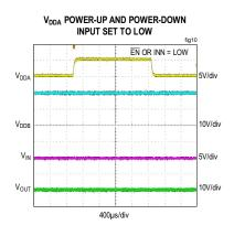
Figure 10. V<sub>DDA</sub> Undervoltage Lockout Behavior (Input Low)
