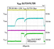
Figure 11.  $V_{DDB}$  Undervoltage Lockout Glitch Filter, UVLO Not Triggered
