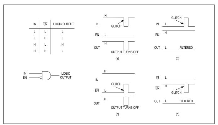
Figure 6. MAX2270\_E Single-Ended Input with Enable
