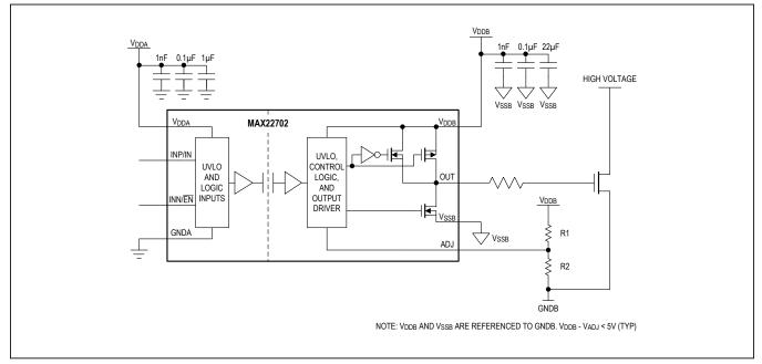
Figure 13. Example Circuit for MAX22702 Adjustable UVLO
