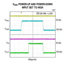
Figure 7. V<sub>DDB</sub> Undervoltage Lockout Behavior (Input High)
