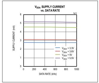
Figure 14. V<sub>DDA</sub> Supply Current vs. Data Rate (typ)
