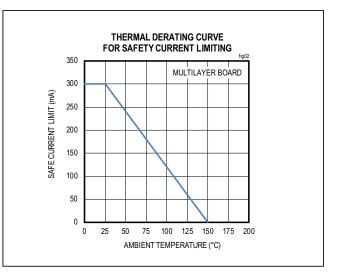
Figure 2. Thermal Derating Curve for Safety Current Limiting
