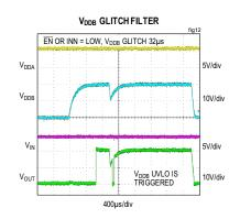
Figure 12. V<sub>DDB</sub> Undervoltage Lockout Glitch Filter, UVLO Triggered
