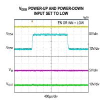
Figure 9. V<sub>DDB</sub> Undervoltage Lockout Behavior (Input Low)
