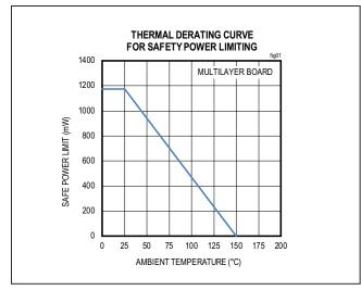
Figure 1. Thermal Derating Curve for Safety Power Limiting
