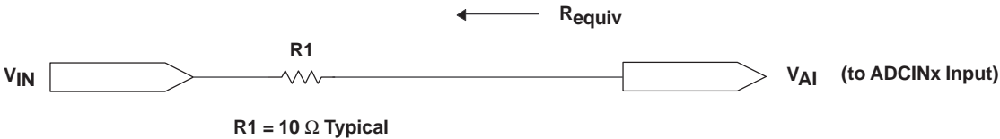
Figure 41. Typical ADC Input Pin Circuit
