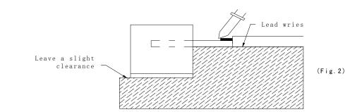
Regarding tinning the leads, compound made of tin ,copper and sliver is proposed with the temperature of  $260^{\circ}$ C. The proportion of the alloyed solution is 95.5% tin, 3.5 % copper, 0.5% silver. The time of tinning is 3 seconds.
