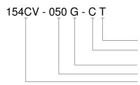
Vent (T = Tube, Blank = No Tube) Electrical (C = Ribbon Cable with Connector, R = Ribbon Cable)
