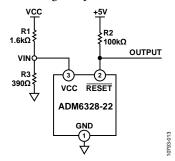
Figure 13. VCC Detection Circuit
