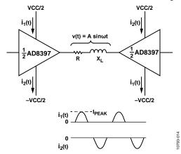
Figure 14. Equivalent Circuit for Calculating Power Supply Current
