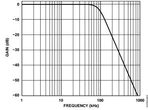
Figure 3. AD8692 Third-Order Low Pass Filter Response
