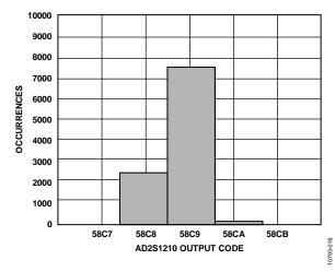
Figure 16. Histogram of Output Codes, 10,000 Samples, Hysteresis Disabled,12-Bit Angular Accuracy Mode, 16-Bit ADC Resolution
