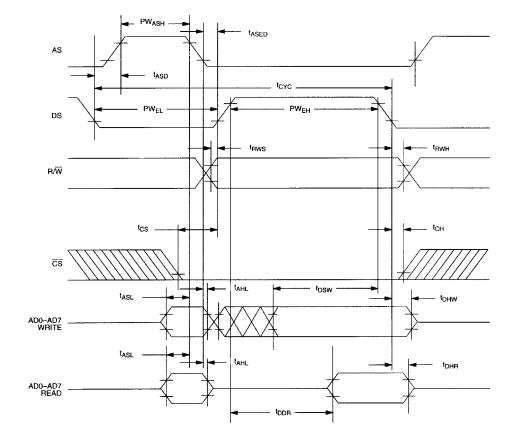
Figure 6. BUS TIMING FOR INTEL INTERFACE WRITE CYCLE
