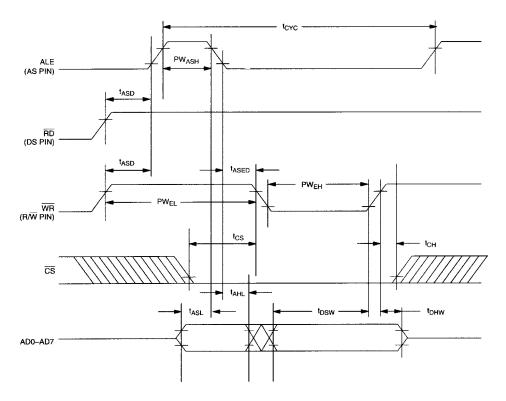
Figure 7. BUS TIMING FOR INTEL INTERFACE READ CYCLE
