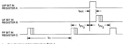
$t_{Pl}$  = Periodic interrupt time interval per Table 1.  $t_{BUC}$  = Delay time before update cycle = 244  $\mu s$ .
